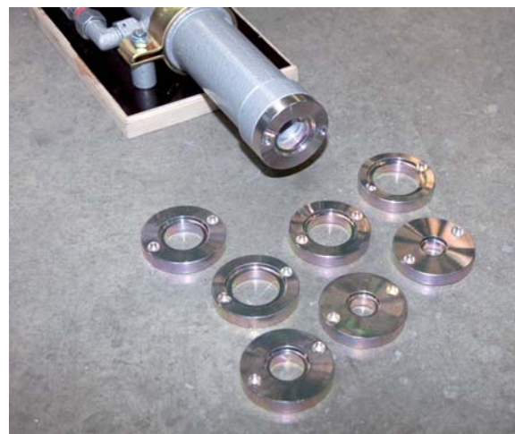
Fig.: Different centering rings to suit different anchor grip diameters
